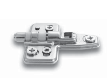
Metal cruciform mounting plate. Knock-in fixing with dowels Ø10mm. Independent vertical adjustment with CAM.
