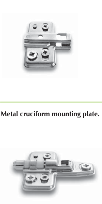
Metal cruciform mounting plate. Knock-in fixing with dowels Ø10mm. Independent vertical adjustment with CAM.
