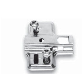
Asymmetric mounting plate for central panel. Fixing by dowels and premounted selftapping screws. Vertical adjustment.
